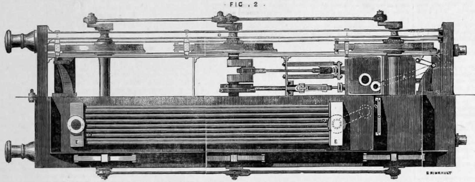
The main object of this invention, by Archibald Sturrock, Locomotive Superintendent of the Great Northern Railway. Doncaster, is to utilise the adhesion derived from the weight of the tender as a power to propel the train in addition to that of the engine proper instead of the engine, as under present circumstances, having the dead weight of the tender to draw.
